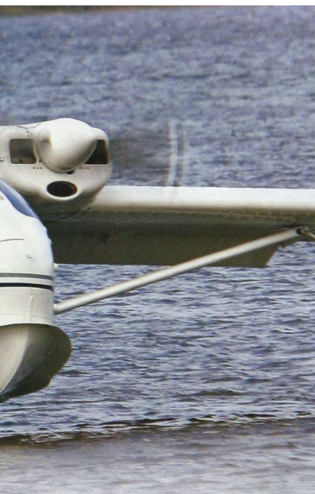
The bulbous bow incorporates a 'docking door' on the starboard side.
