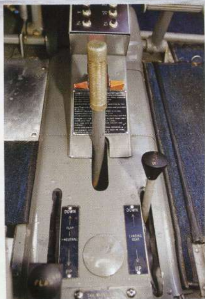
The flap and undercarriage selectors are on either side of the hydraulic hand pump.
