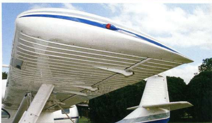
The taxi and landing lights are in the port wing's leading edge.
