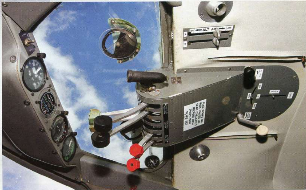
Above: The throttles, propeller levers and mixture controls are all located in the roof, along with the rudder and elevator trimmers, trim position indicators and alternate air selectors.
