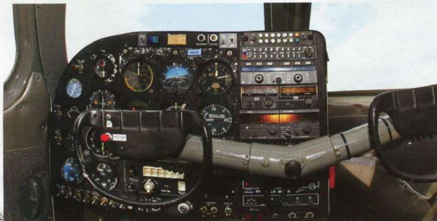
The flap and undercarriage selectors are on either side of the hydraulic hand pump.
