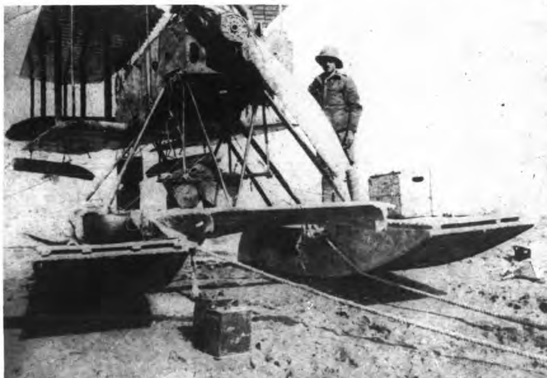
A Short 184 at Orah with food drop gear fitted for relief of the Kut al Amarah siege. :R. Vann
