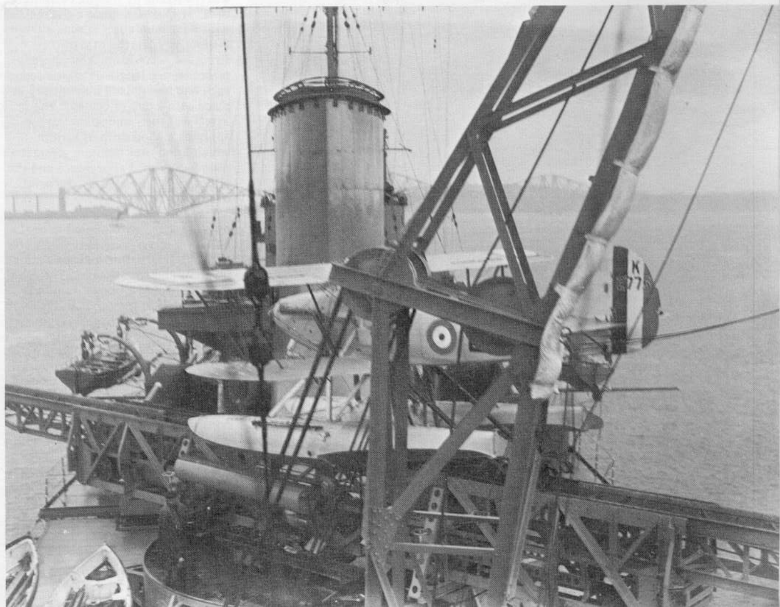
Above: views of extending sections. Below: the Osprey photographed just as it is racing down the catapult during launch. Almost the full extended structure is seen here. The Forth Bridge is in the background. Flight International 10870S
