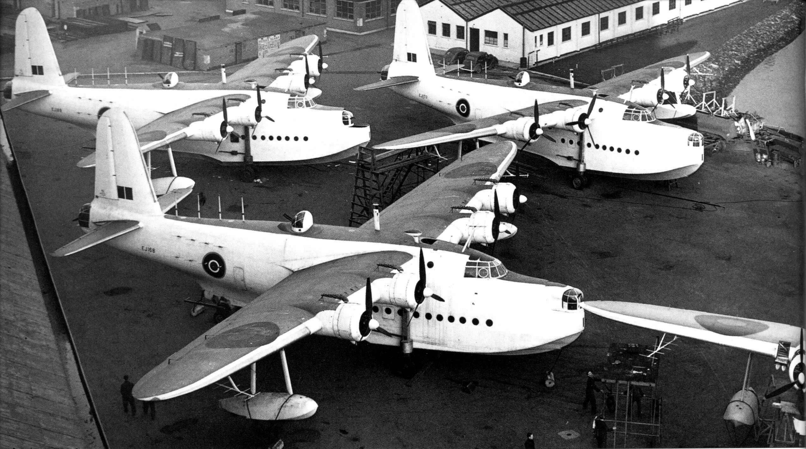
Factory-fresh Mk IIIs EJ168, EJ169 and EJ170 sit on the slipway at Belfast. Each is fitted with the ASV Mk II 'stickleback' antenna array on the top and side of the rear fuselage, and the Yagi direction-finding gear under the wings and above the cockpit. The Pegasus Mk XVIII engines of this batch have the long flame-dampening exhaust pipes. Others had much simpler exhausts.
