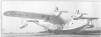
Three views of the Knackleduster showing different wing float mountings: Top , the intermediate inserted-use struts with spring diagonal; right , the original side single strut with wire cross-bracing; and below , the final single strut mounting retaining the spring diagonal.
