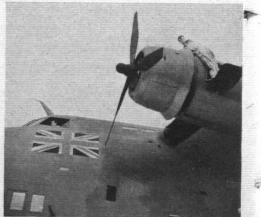
The engines of the Bristol are accessible in flight, and small platforms make overhaul on the ground easier. The view on the left shows the bows, with the forward door for the crew.
