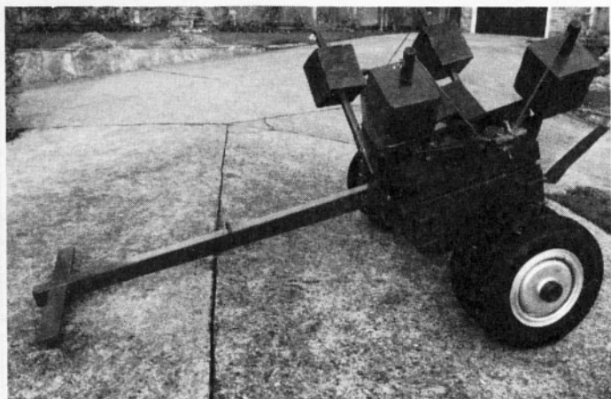
Sunderland type tail trolley. Manufactured by Captain Vic Hodgkinson for 'Beachcomber', Southampton Hall of Aviation. (Captain Vic Hodgkinson)
