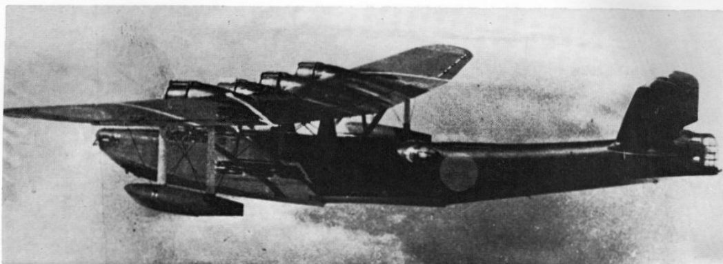
An H6K4 in flight with bombs attached to the wing support struts. The drab Pacific War colour scheme was introduced in mid-1942 for all combat aircraft of the IJNAF.
