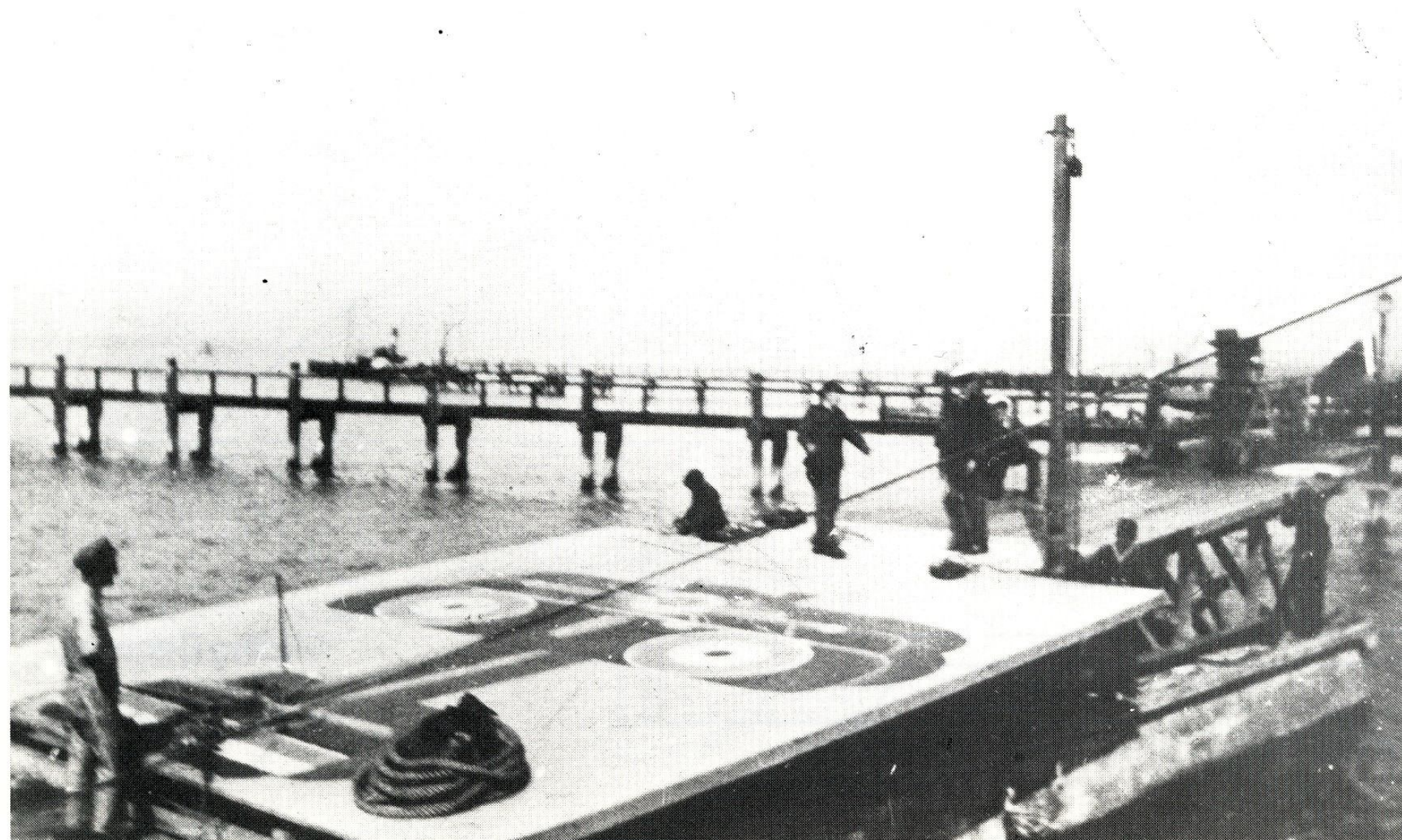
Lighter with modified take off platform for a Sopwith Camel. Note painted outline of aircraft plus shadow on the deck. It could be that this was meant to create the impression that a Camel was aboard the lighter after it had in fact taken off. Bearing in mind the height at which Zeppelins operated this might have been a practical deception.
